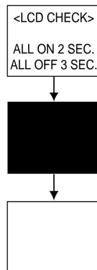
6. The test repeats itself. To stop the test, turn the power switch off and on again.
