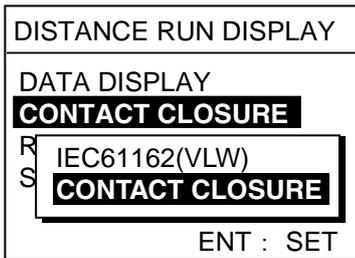
4. Press ▲ to select IEC 61162(VLW) and press the [ENT] key.
