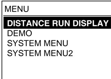
2. Press the Omnipad at ▲ or ▼ to select a menu item (current selection is highlighted) and press the [ENT] key. For example, when DISTANCE RUN DISPLAY is selected the following display appears. Distance run is a form of contact closure, 200 pulses/nm. To select IEC 61162 sentence, see paragraph 1.6.1.
