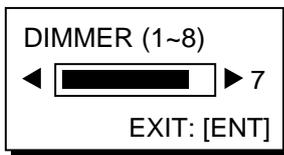
2. Press the Omnipad at ◀ or ▶ to adjust the dimmer. The setting range is 1 to 8 and the default setting is 4.
