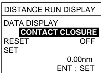
3. Press the Omnipad at ▲ or ▼ to select the menu item desired and press the [ENT] key. For example select RESET.
