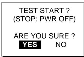
4. Press the [ENT] key to start the test. In a few moments the display should change as shown at the top of the adjacent column.
