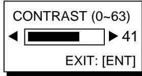
2. Press the Omnipad at ◀ or ▶ to adjust the contrast. The setting range is 0 to 63 and the default setting is 48.
