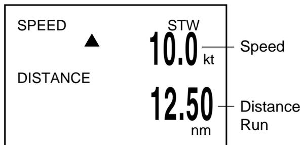
**Note:** STW means Speed Through Water. This indication flashes when transducer temperature, which can be monitored on the TEST display (see page 16), is abnormal. This means speed accuracy is less than stated in the specifications.
