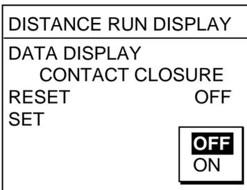
4. Press the Omnipad at ▲ or ▼ to select the menu option desired and press the [ENT] key.
