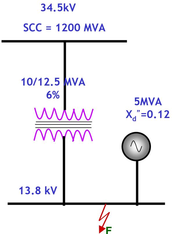
Calculate the fault current at F
