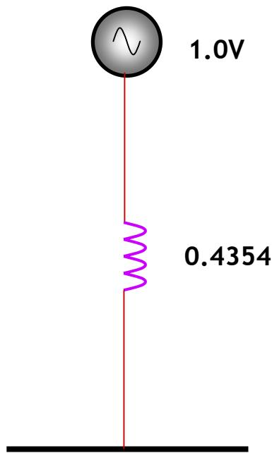
$$I_{Fpu} = \frac{V_{pu}}{Z_{Eq}} = \frac{1.0}{0.4354} = 2.297 \text{ pu}$$
