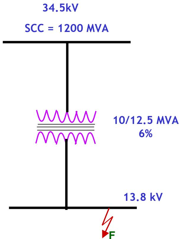
Step 3: Calculate fault current
