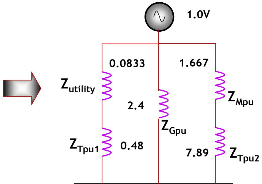
Calculate the fault current at F
