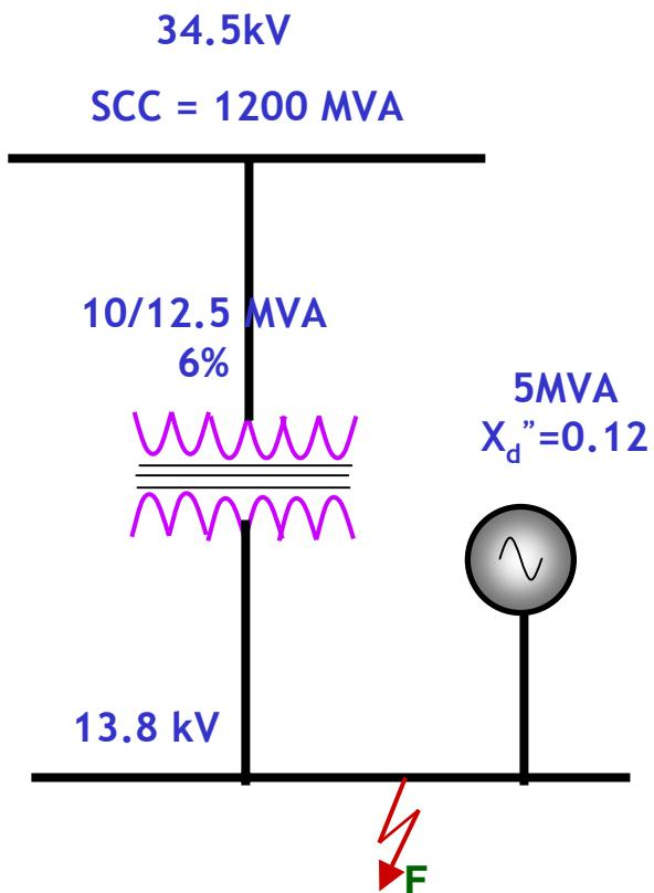
$$Z_{\text{utility}} = \frac{\text{MVA}_{\text{base}}}{\text{MVA}_{\text{oldbase}}} \times \frac{\text{kV}_{\text{oldbase}}}{\text{kV}_{\text{base}}}$$
