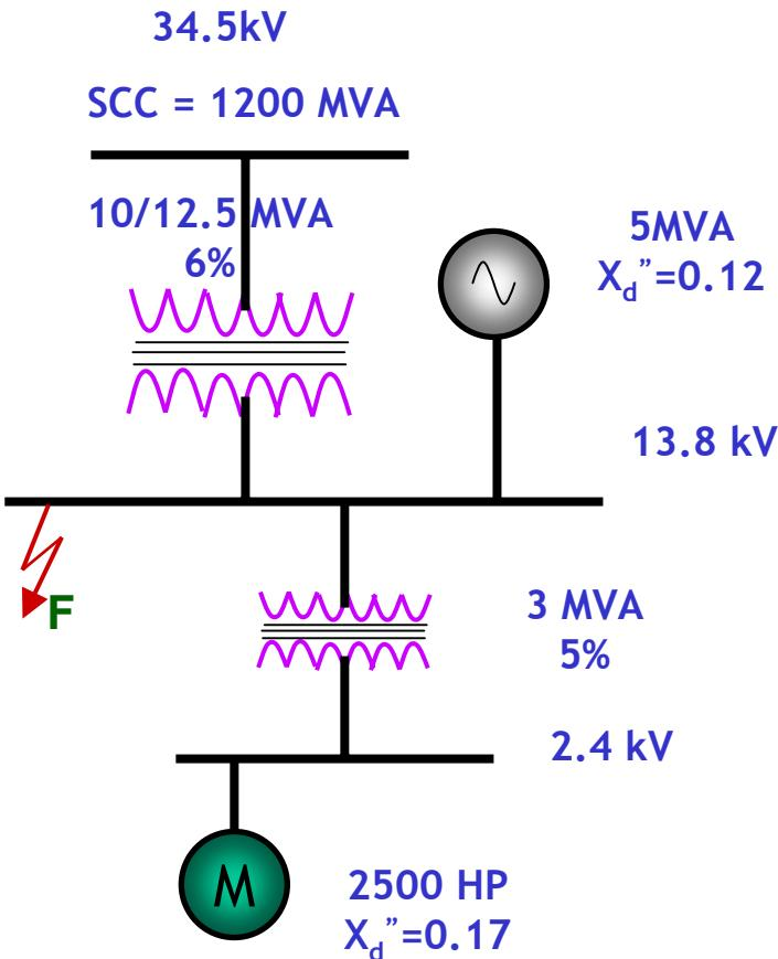
$$Z_{\text{utility}} = \frac{\text{MVA}_{\text{base}}}{\text{MVA}_{\text{oldbase}}} \times \frac{\text{kV}_{\text{oldbase}}}{\text{kV}_{\text{base}}}$$
