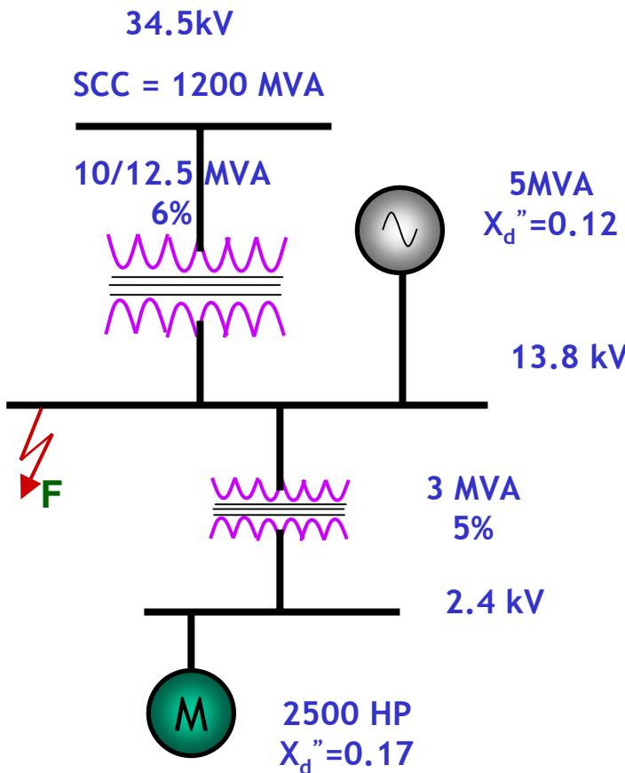
Calculate the fault current at F
