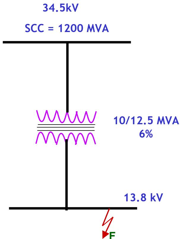
Step 3: Calculate fault current
