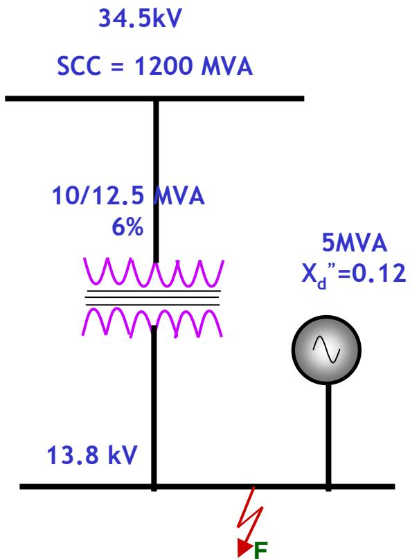
Calculate the fault current at F
