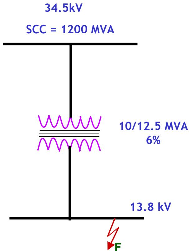
Calculate the fault current at F
