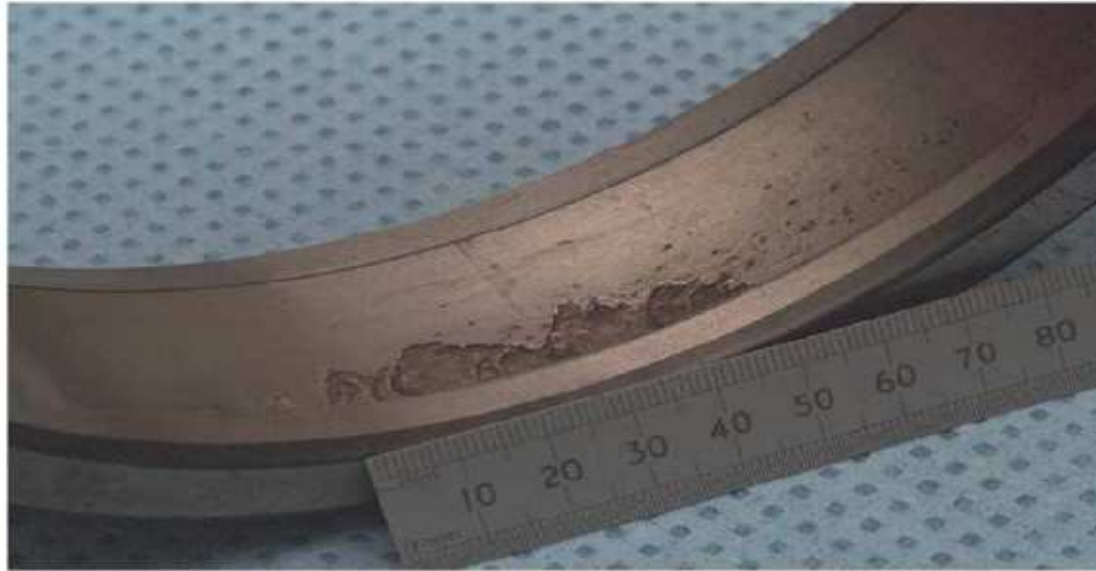
Figure 4 - Photograph showing bearing outer race damage
