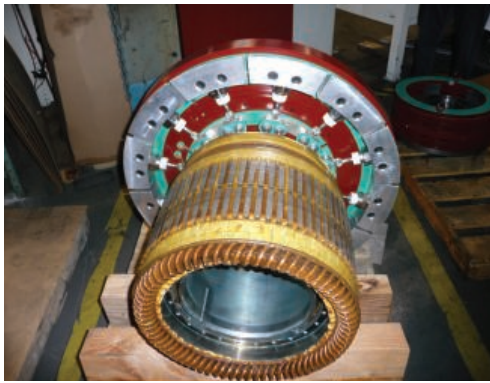
Top row (L to R): Rotating rectifiers with armature; Stationary exciter field
