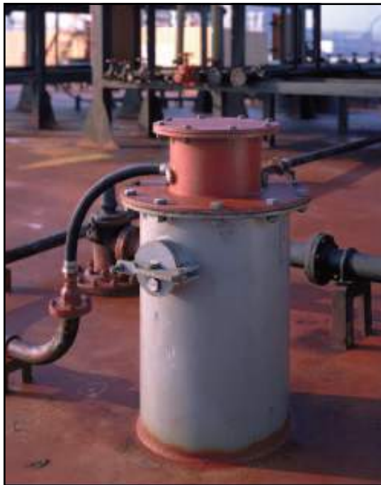
The Parabolic Antenna Transmitter installed on deck before painting.
