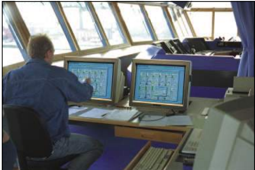
The photo shows two Saab TankRadar MaC Work Stations placed on the bridge.
